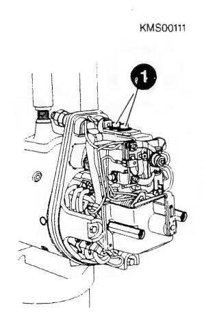
Disassembling control relay and starting-motor solenoid
